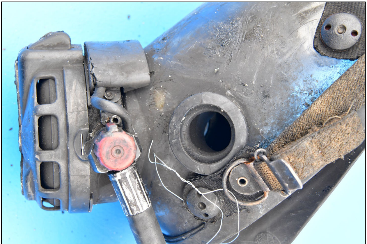
Figure 56. Facepiece attached to the regulator of E257's back-up position SCBA worn by Firefighter Timothy Klein.
