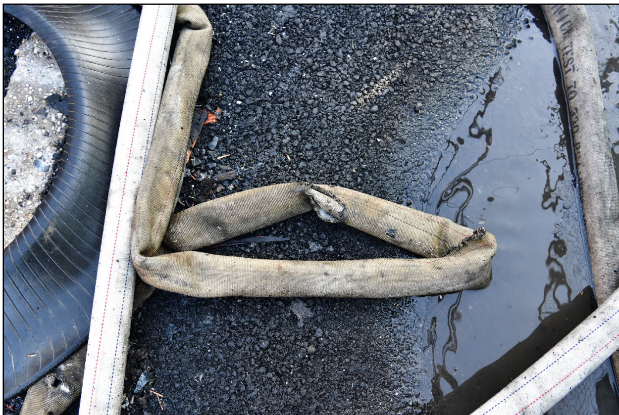
Figure 36. E257's hoseline with burns that caused a burst length.
